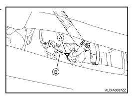
4. Tighten the PNP switch bolts (A).
