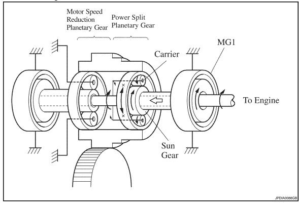
Motor Speed Reduction Planetary Gear
