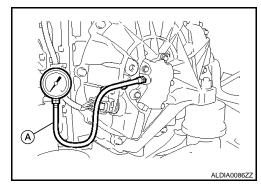
3. Remove the suitable tool and install the fluid pump cover plug with a new O-ring and tighten to the specified torque.
